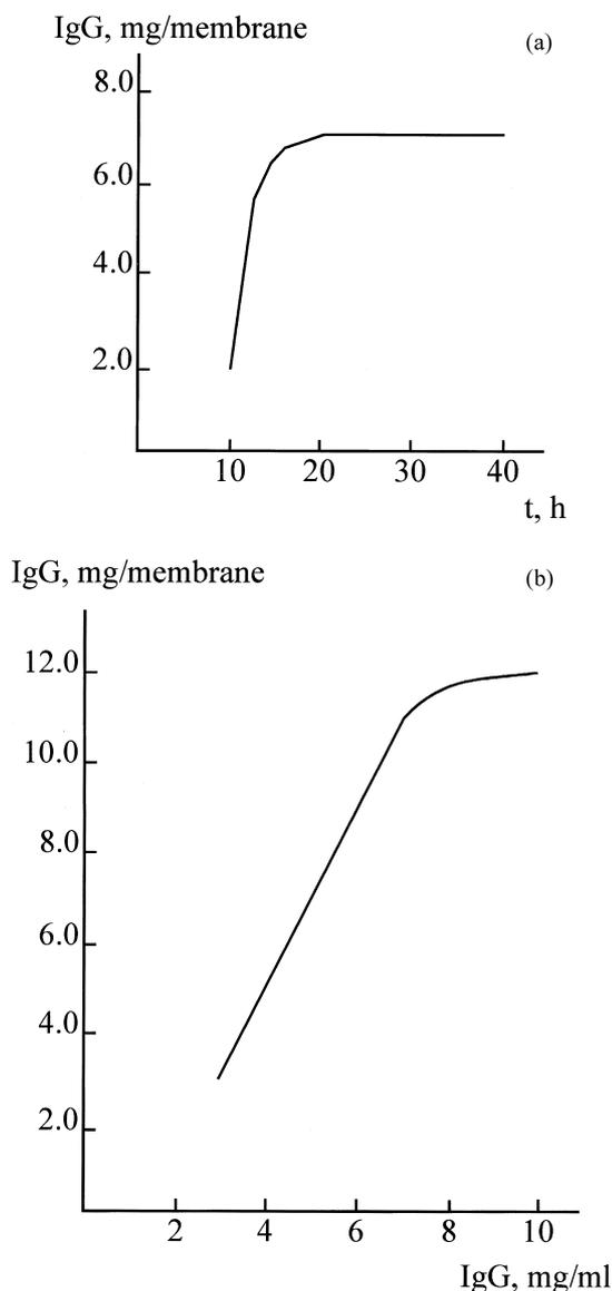
Fig. 3. (a) Dependence of the amount of hIgG bound to the GMA-EDMA disc (25×2 mm) on the reaction time. Conditions: sodium carbonate buffer, pH 9.3; 30 ml of 5 mg/ml Protein G; temperature 30°C. (b) Influence of IgG concentration on the hIgG amount immobilized. Conditions: dimensions of disc, buffer and temperature were the same as in (a); the time of reaction was 16 h.
