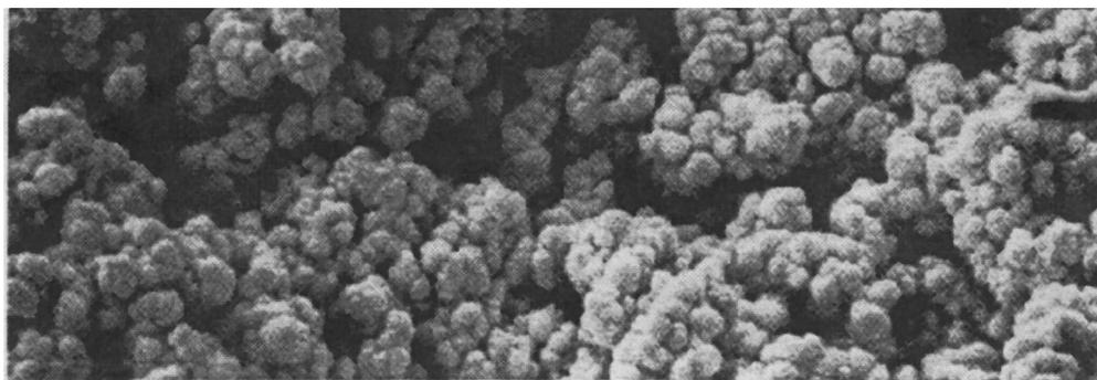
Fig. 1. SEM picture of GMA–EDMA polymer macroporous structure.
