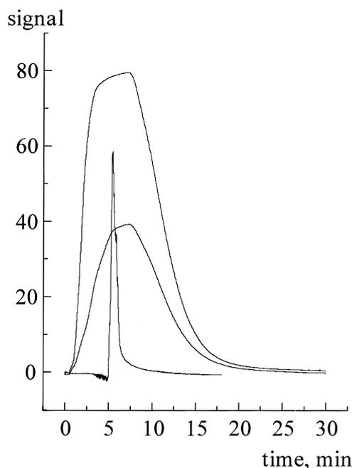
Fig. 5. Frontal analysis of Protein G capacity. Conditions: CIM disc, flow-rate, 1 ml/min; sample volume, 5 ml (loop); total amount of Protein G in sample loaded, 0.83 mg (lower curve) and 1.67 mg (upper curve); 0.18 mg were desorbed in both cases (one sharp peak which means the same quantity of desorbed Protein G). Mobile phase of adsorption step is PBS buffer, pH 7; desorption was carried out with 0.01 M HCl, pH 2.0.
