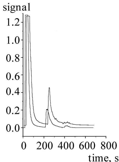
Fig. 6. Fast isolation of Protein G from 1:5 and 1:10 diluted cell lysate (solid and dotted elution curves, respectively). Conditions: buffer A (adsorption) was PBS, pH 7.0; buffer B (desorption) was 0.01 M HCl, pH 2.0; flow-rate, 3 ml/min; CIM disc; probe volume, 5  $\mu$ l. Stepwise gradient: 0–2 min, 100% A; 2.0–2.1 min, 0–100% B; 2.1–6.0 min, 100% B; 6.0–6.1 min, 100–0% B; 6.1–10.0 min, 100% A.
